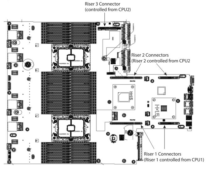
Figure 9 shows the locations of the PCIe riser connectors on the C240 M6 LFF motherboard.
