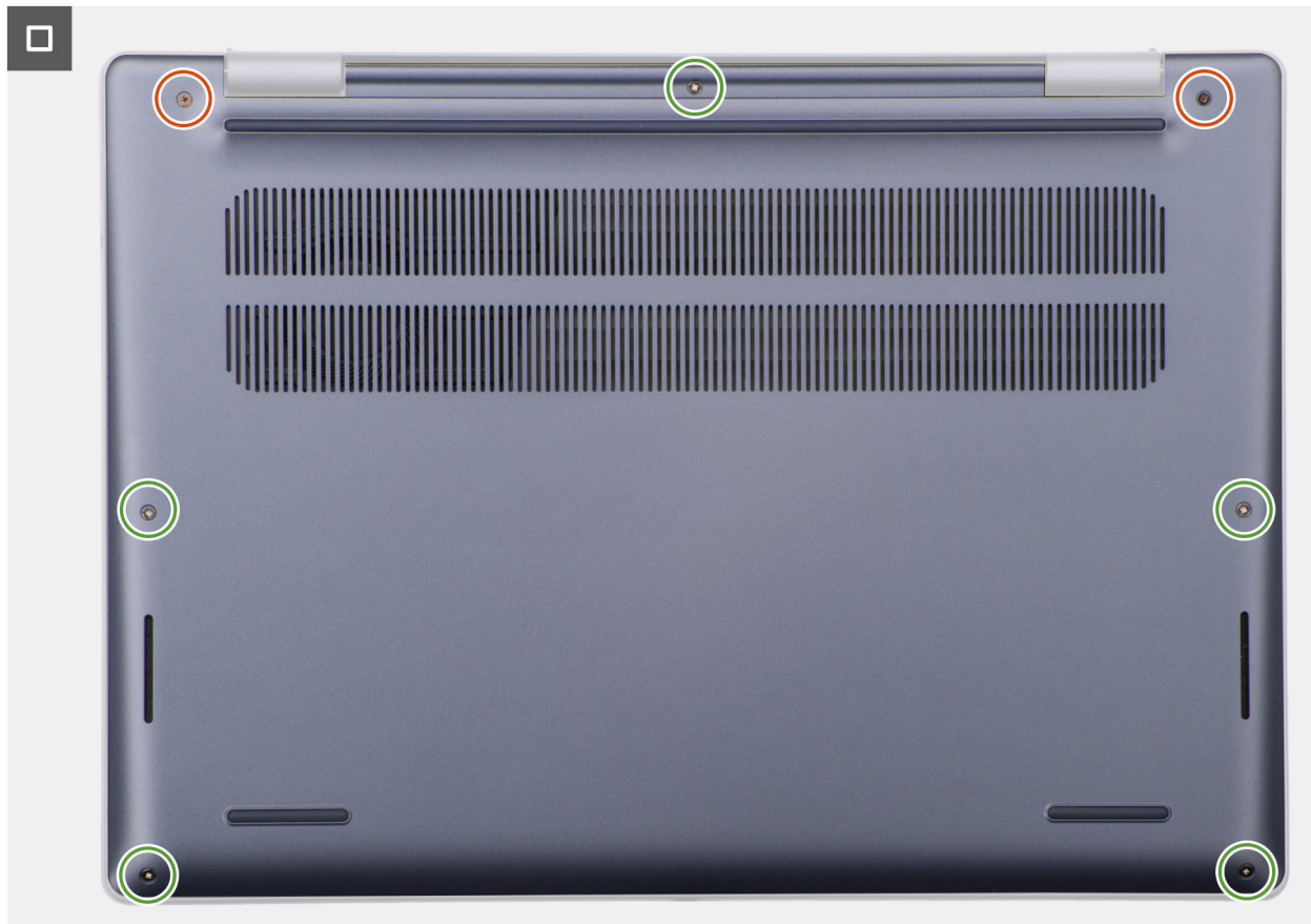
Figure 19. Installing the base cover
