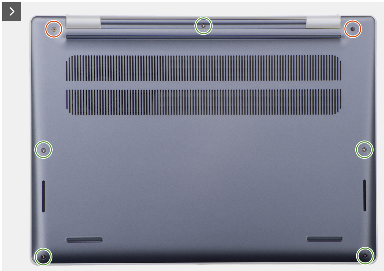
Figure 16. Removing the base cover
