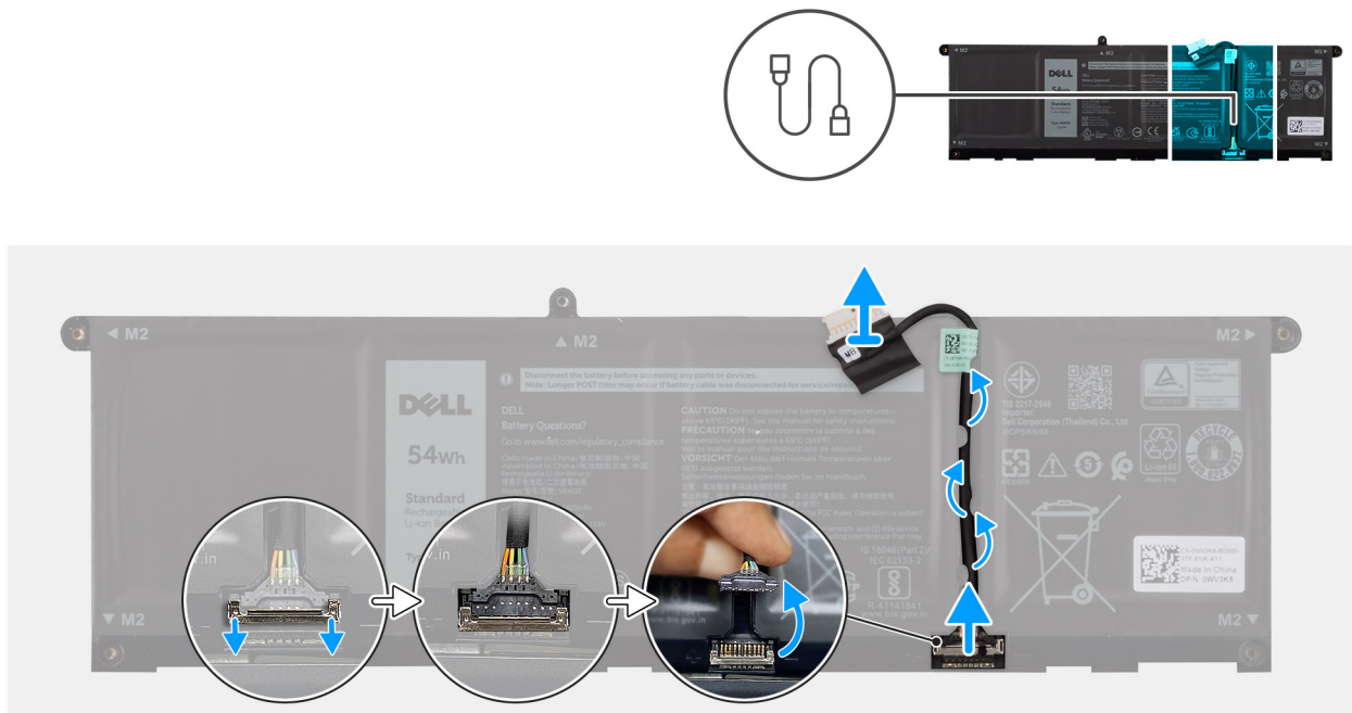
Figure 26. Disconnecting the battery cable
