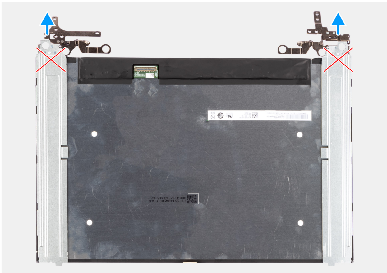
Figure 80. Removing the display panel
