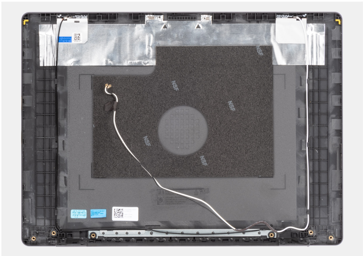
Figure 89. Display back-cover and antenna assembly
