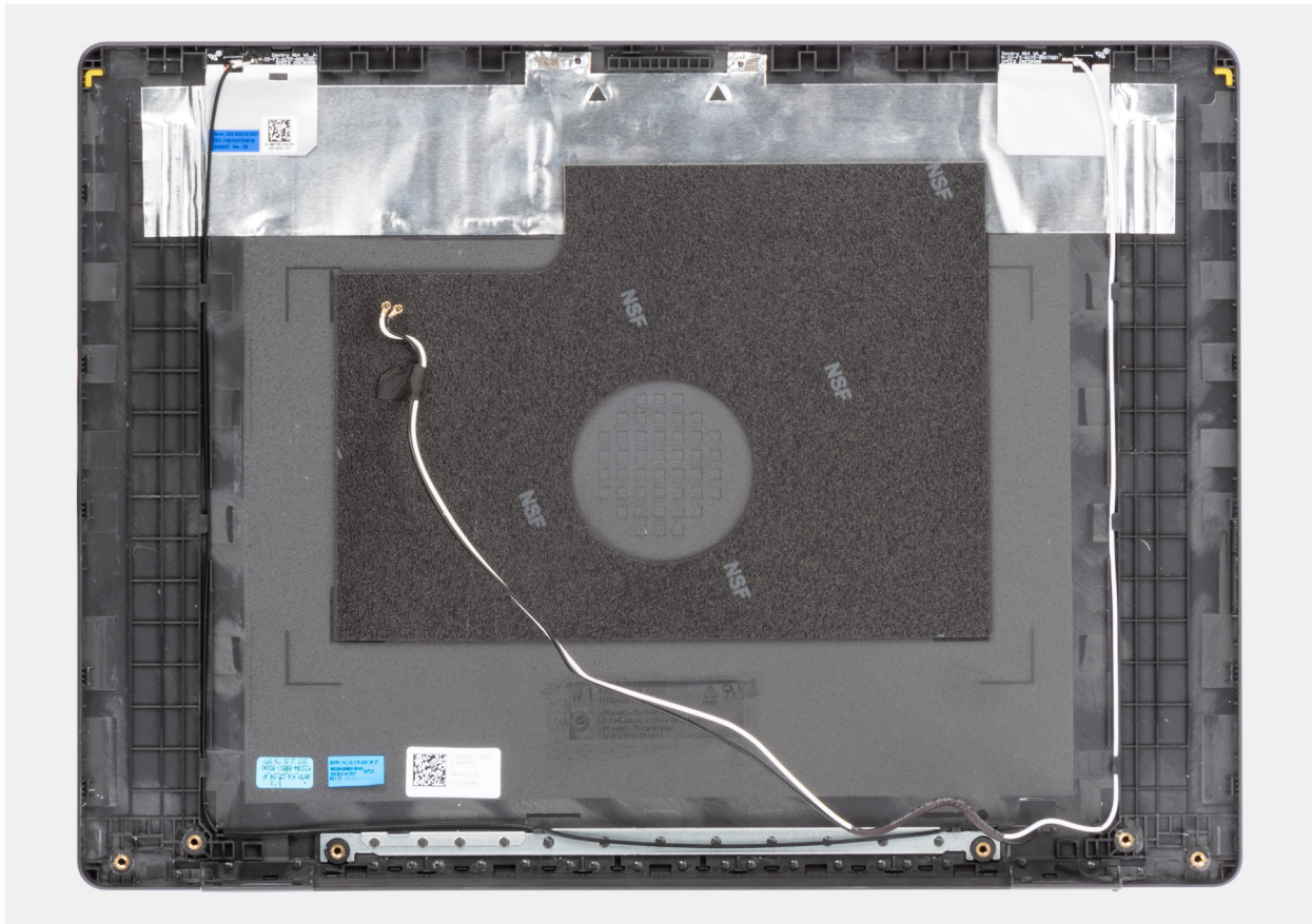
Figure 90. Display back-cover and antenna assembly
