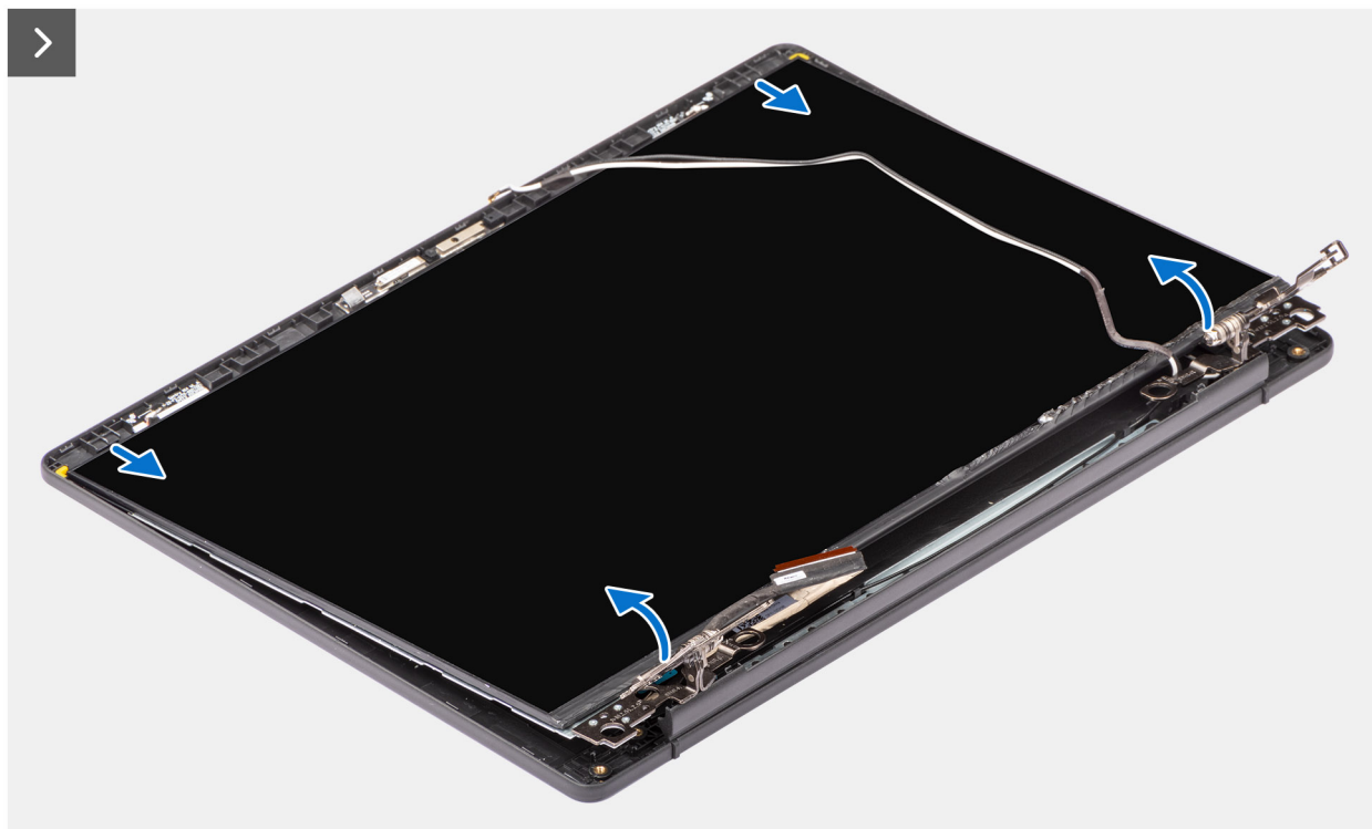
Figure 78. Removing the display panel
